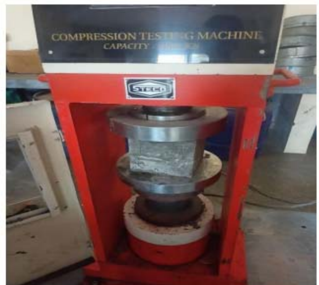
Compressive test on cubes
